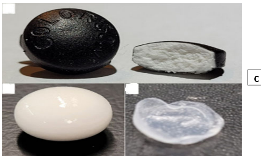
Figure 3: Tablets coated with CMS after immersion for 15 min in SGF containing Lugol-Iodine solution (A), after 2 h in SGF (B) and the remaining shell (C).
